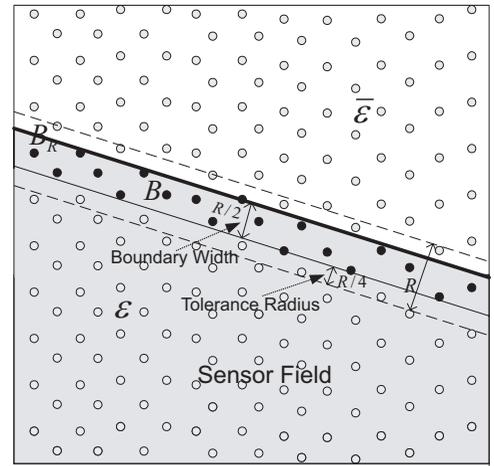
Fig. 4. An illustration of boundary model with  $r = R/4$ .
