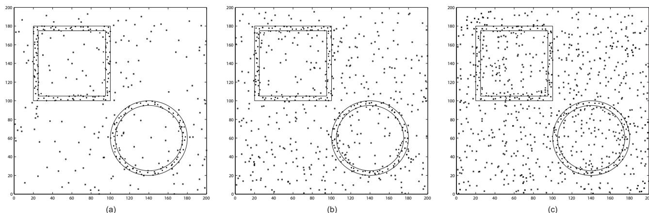
Fig. 6. Simulation results: left)  $e_f = 85\%$  with  $p_c = 5\%$ ; middle)  $e_f = 79\%$  with  $p_c = 12.5\%$ ; right)  $e_f = 60\%$  with  $p_c = 25\%$ . And  $p_f = 2.5\%$  in all three cases. '\*' denotes the detected boundary nodes, and '□' denotes compromised and faulty nodes.
