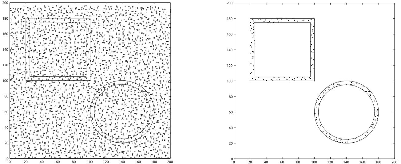
Fig. 1. The left figure denotes a sensor field, where the event area is located inside the outer square and circle. In the figure, normal nodes are denoted as ‘o’, compromised and faulty nodes are denoted as ‘□’. The right figure is an illustration of boundary  $\mathbb{B}$  with  $r = \frac{R}{2}$ . By definition, the nodes denoted as ‘\*’ are the boundary nodes.
